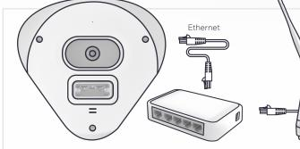
Install your camera and plug it into a PoE switch to power it up.
